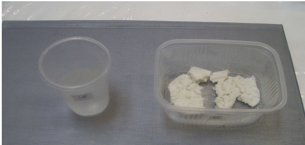
Fig. 3 The appearance of solidified specimen after water has been added. (Solution HNO 3 , 0,5M, # 15 in Table. 3.)
