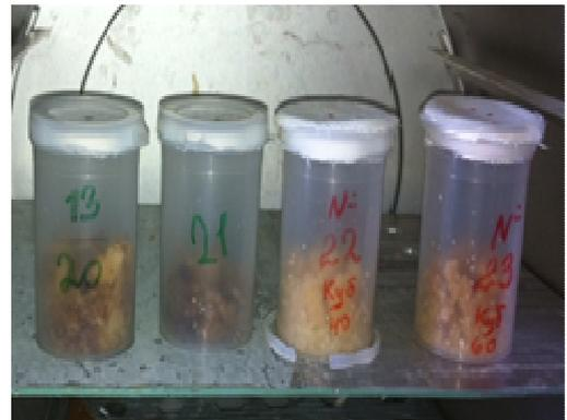
**Figure 9. Solidified aqueous waste samples.**
