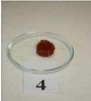
**Figure 10. Solidified sample of the iron-containing precipitate from decontaminating LRW by coagulation.**
