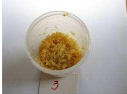
**Figure 4. Sample appearance after solidification of vacuum oil**
