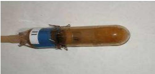
**Figure 8. The appearance of specimen (polymer N910 +oil+TBP) after irradiation.**
