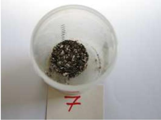
**Figure 3. Sample appearance after solidification from waste tank organic residue**
