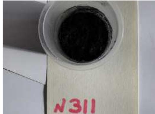
**Figure 6. Specimen after solution solidification with schungite included**
