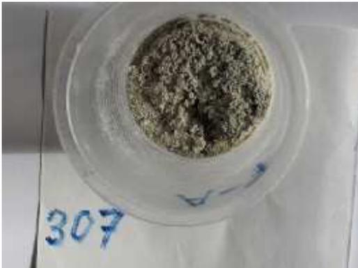
**Figure 5. Specimen after solution solidification with zeolite included**
