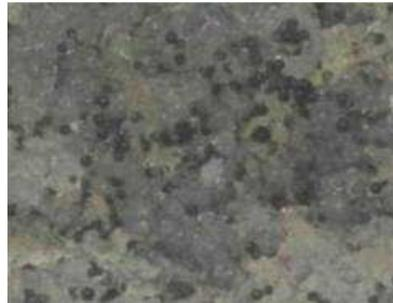
**Figure 11. A sample of the solidified S957 resin saturated with uranium.**
