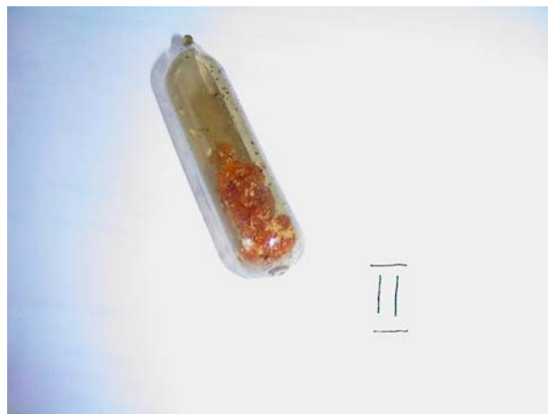
Picture 7: Irradiated Sample at 77,000,000 Rad
