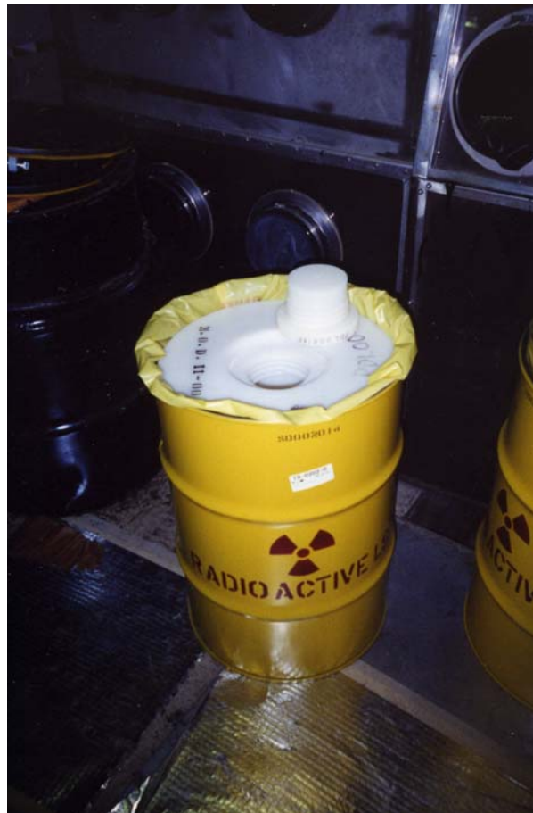
Picture 1: Polyethylene Drum for Tritiated Oil
